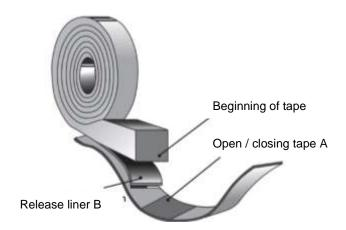
3) Press adhesive side of tape onto clean window frame tightly. Beginning and end of tape have to be joint with an over length of 10-20 mm.
