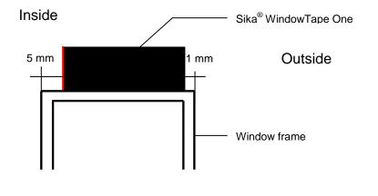
4a) in case the tape is mounted in one piece around the frame (joint less edges) than the mounting of the tape starts on the frame upper / top side.
