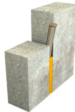
Fire resistant backer rod and standard joint sealant
