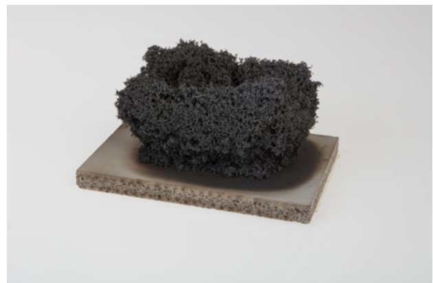
Highly intumescent, fire resistance wrap before (top) and after (bottom) exposure to heat
