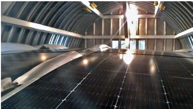
Wind uplift test with east-west oriented SSM2.
