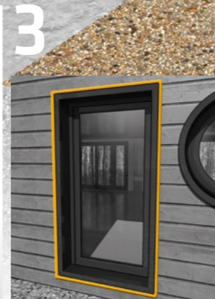
2 Peripheral sealing of doors, windows and joinery
