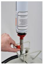
4. Check the tap on the assembly is off before applying the Sika Spray Cleaner. Screw the Sika® Spray Cleaner canister into the top of the assembly and open the red valve.
