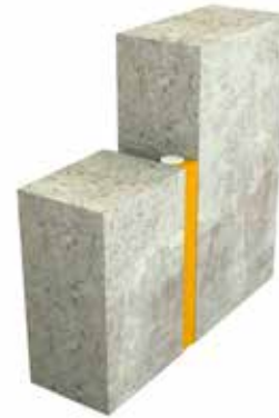
PE backer rod and fire resistant sealant
