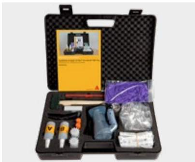
The Sika qualitative Color Test Kit for penetration depth testing.
