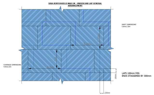
All vertical lap joints are sealed with Sika BentoShield SS50 Bonding Tape. Where accessible externally (ie. applications to be backfilled) this can be applied externally to the PE layer.
