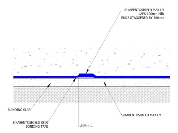
SikaBentoShield Max LM membrane should be applied inside the formwork, prior to the casting of concrete, to facilitate the fully-bonded property of the SikaBentoShield Max LM membrane to the concrete. Care shall be taken when striking the formwork, to prevent undue damage to the fully-bonded SikaBentoShield Max LM.
