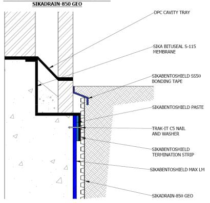
Backfill material shall be of compactable soils and free of construction debris. Backfill shall be clean, well graded and compacted every 300mm to 85% modified proctor (as defined by ASTM 1557) and meet these general specifications:
