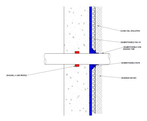
Terminate SikaBentoShield Max LM at ground level, etc., integrating the SikaBentoShield Max LM with a damp-proof course/cavity tray (as per architects arrangement), by extending the DPC to overlap SikaBentoShield Max LM a minimum of 150mm. The SikaBentoShield Max LM /DPC lap should be closed by a 5 x 50mm fillet of SikaBentoShield Paste placed central inside the lap. The whole lap is then secured using SikaBentoShield Termination Strip.
