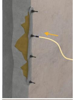
...continue this procedure until the crack is completely full.
