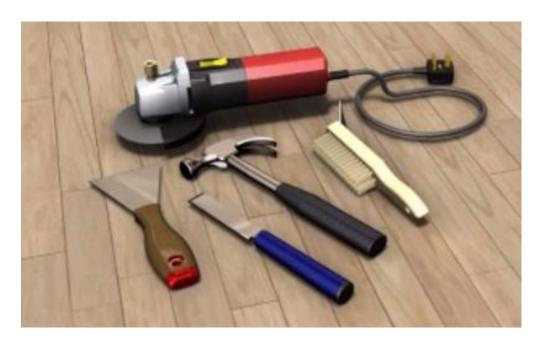
Use appropriate tools for substrate preparation or to fully remove all injection ports and Crack Sealing material and Injection ports.
