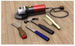
Use appropriate tools to fully remove all injection ports and Crack Sealing material
