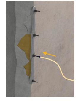
...disconnect the injection cartridge from the first port and reconnect to the second port and inject until resin flows from the third port....
