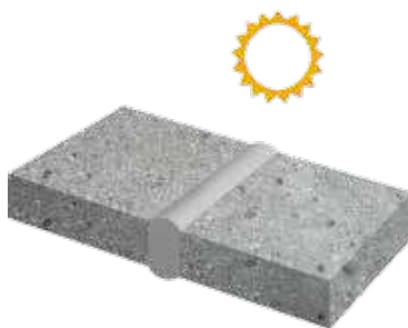
Expansion of building elements
