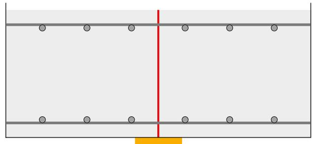
The positioning of the waterstop should be appropriate for the method of construction and the risk level.
