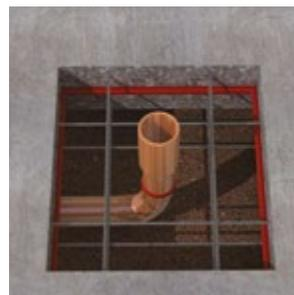
Waterproofing details are required at all types of penetrations. The SikaSwell® system using sealants and different-sized profiles can meet many different requirements.
