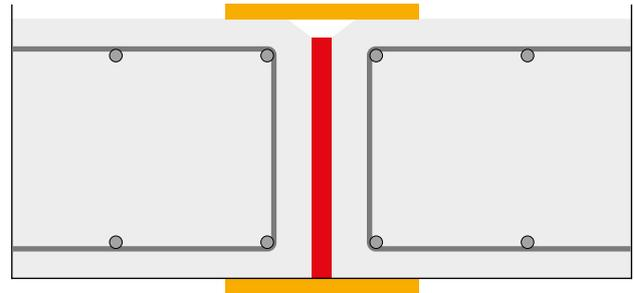
Where internal waterstops are used, correct fixing is essential to keep the waterstops in place during the concreting operations. Good compaction of the concrete around the waterstops is also necessary to avoid paths for water ingress.
