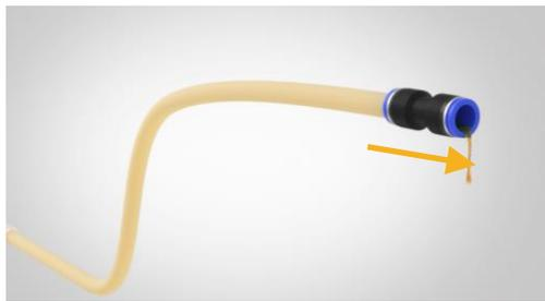
Extrude a quantity of resin to waste to ensure an even homogeneous mixture
