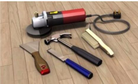
Use appropriate tools to fully remove all injection ports and Crack Sealing material
