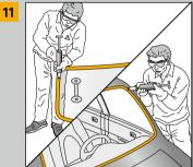
■ Apply a triangular bead glass or the aperture
