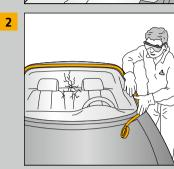
Cover the aperture with masking tape
