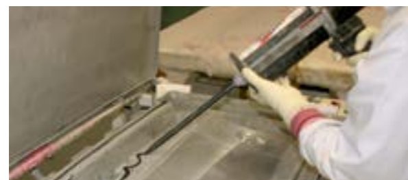
Bonding of SMC parts with Adekit A280.
